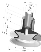
1.5 Bellows Suction Cup Series 8A Ø 49MM
